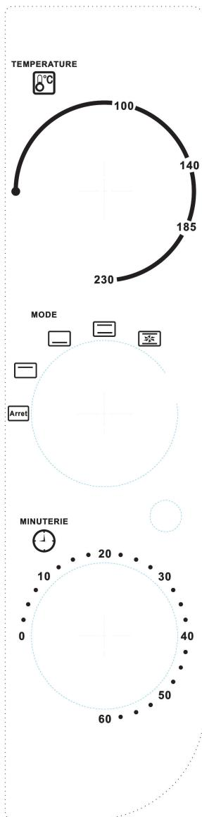
**Temperature Knob:** the temperature choice is from low to 230°C. You could select desired temperature according to the practical situation.
