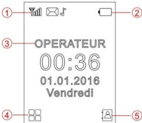
1. **Signal Bar:** It indicates the signal strength. Four bars indicate optimum reception for your calls.
